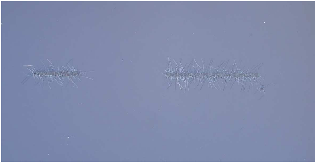
Figure 6.3 InN NWs grown out of 2 nm Au catalyst (catalyst pattern dimensions: 5 \mu\text{m} x 100 \mu\text{m} and 5 \mu\text{m} x 200 \mu\text{m} ).
