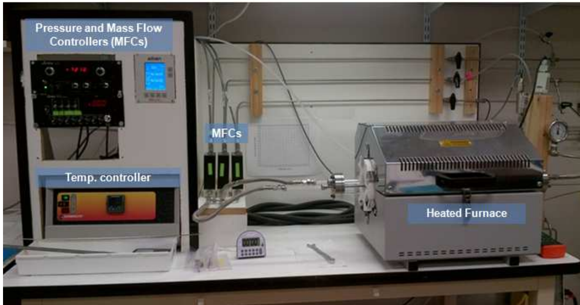
Figure 2.3 CVD system setup, pressure and mass flow controllers (MFCs), MFCs, temperature controllers and heated furnace.
