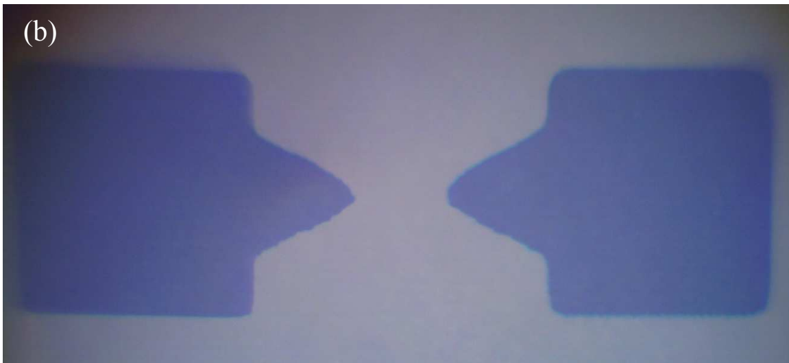
Figure 3.2 Optical images of 2 nm Au pattern. (a) Size of lines is 3 \mu\text{m} \times 30 \mu\text{m} and the diameter of the circles is 3 \mu\text{m} . (b) The size of the patten is 50 \mu\text{m} \times 50 \mu\text{m} .
